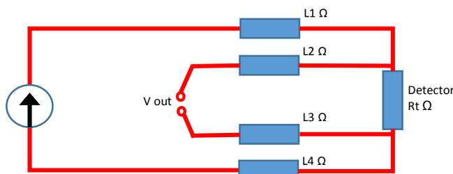
One pair of lead wires takes the constant current power source to the detector and the other pair is used to measure the actual voltage drop across the detector. Therefore by using a constant current source and being able to simply measure the change in voltage across the PT100 detector rather than a change in resistance (Ohms Law), any fixed or varying lead wire resistance is totally eliminated.
