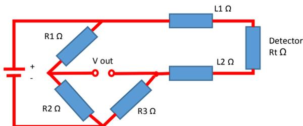
Where the lead lengths are short, and where they are exposed to the same temperature as the detector, then in theory this can be accounted for.
